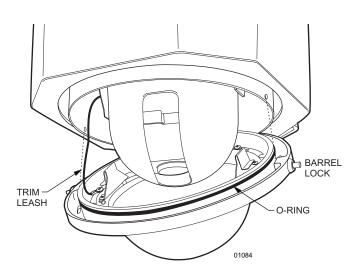
b. Align barrel locks in lower dome with the holes located on each side of the back box. Push lower dome onto back box. Press the pins of the barrel locks IN to secure the lower dome.
